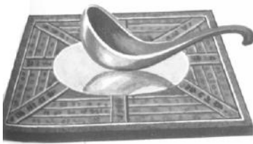
Left: A Chinese spoon compass. A spoon shaped piece of magnetic stone, called a loadstone, was placed on a polished bronze board. The spoon turned until it pointed to the North Pole.
